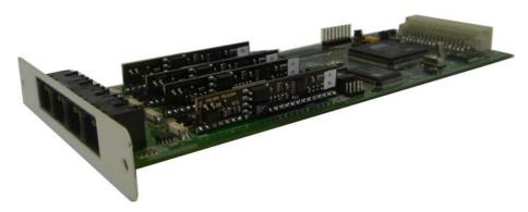
The IPcts AT4 card provides four analogue PSTN trunk line ports to interface to a Service Provider's analogue telephone lines. It has four physical RJ11 interfaces enabling simple installation into the IPcts system application.
